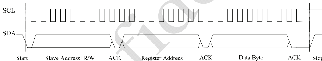
Figure 5: Serial Interface Slave Mode Protocol
